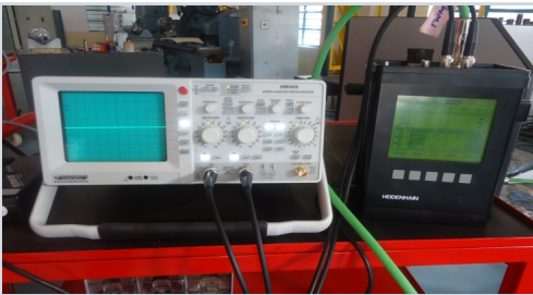
Electronic test and diagnostic equipment supporting encoder, parameter and waveform assessment.
