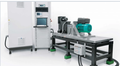
Controlled motor test system for validation, performance checks and post-repair confirmation.
