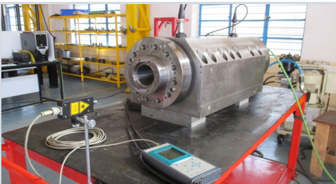
Precision diagnostic setup for alignment, measurement and condition analysis during spindle repair work.
